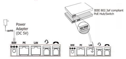
Note: If POE works, the phone doesn't need to connect to the AC power adapter. Make sure the Ethernet cable and switch/hub is POE compliant.
