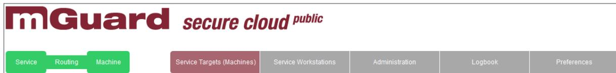
Figure 7.1: Status indicator: Service (VPN tunnel active/inactive) | Routing (performed/not performed) | Machine (available/unavailable)
