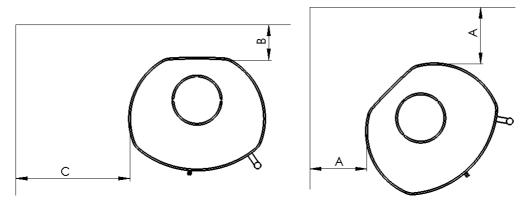
If a non-combustible board is laid under the stove, it must protrude at least 30 cm off in front of the stove and 15 cm off at each side of the fireplace opening.
