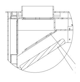
Steel smoke baffle plate Skamol smoke baffle plate
