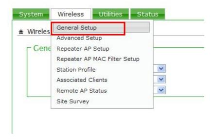
The "general set" interface is mainly to set the wireless frequency band mode and channel:
