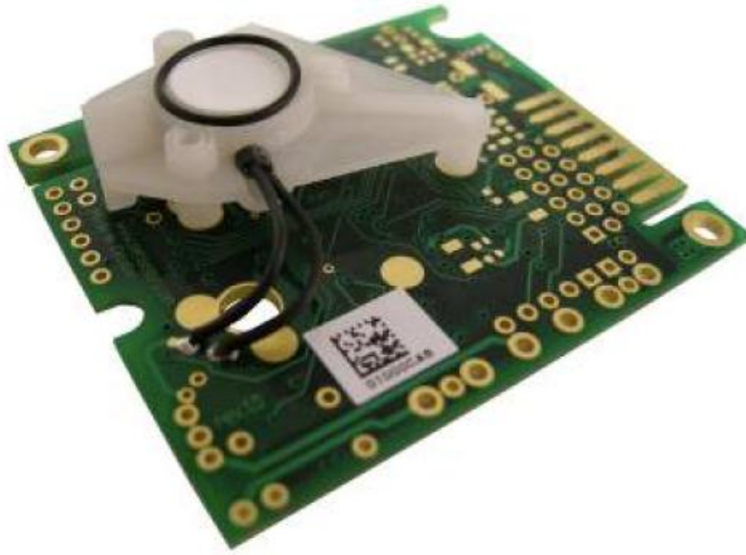
Figure 5. Diffusion model The sensor can be supplied in tube in/out modification with different orientation of tube attachment head in steps of 120 degrees.
