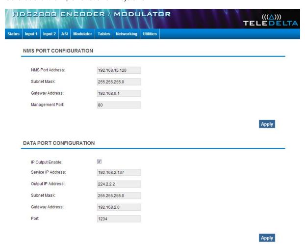
Note: In this example if using VLC, set the VLC network stream to udp://@224.2.2.2:1234 and connect the stream from the **DATA** port – ensure your computers firewall is either disabled or accepting of the above port address
