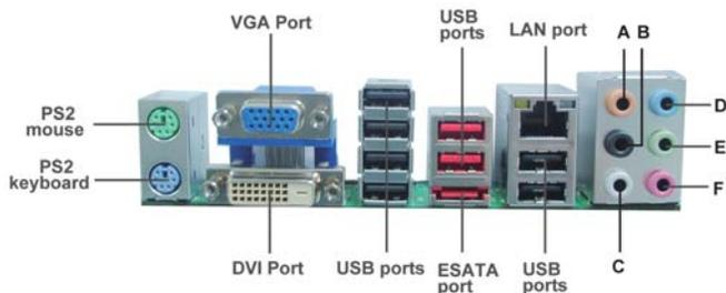
**PS2 Mouse** Use the upper PS/2 port to connect a PS/2 pointing device.
