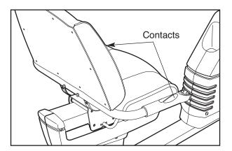
When your pulse is detected, dashes will appear in the display, and then your heart rate will be shown. For the most accurate heart rate reading, hold the contacts for at least 15 seconds. Note: If you continue to hold the handgrip pulse sensor, the display will show your heart rate for up to 30 seconds.
