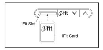
Next, select the desired workout on the iFit card by pressing the increase and decrease buttons next to the iFit slot.
