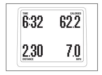
**Speed**—This display will show your pedaling speed, in miles per hour (MPH) or kilometers per hour (KM/H).
