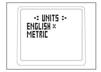
To change the unit of measurement, press the resistance increase and decrease buttons to choose the desired unit of measurement.
