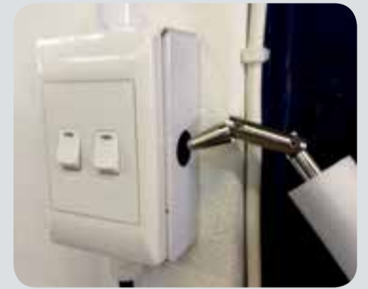
Clear access for test finger – now to test for live parts.
