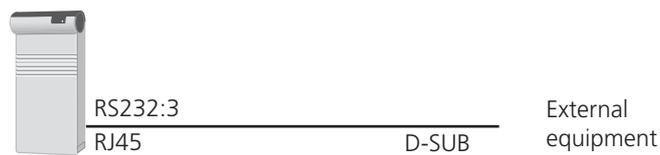
Figure 26. Connection to external equipment.
