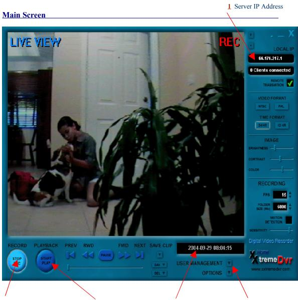
2 Starts/Stops Record Mode 3 Enters/Exit PlayBack Mode 4 Date & Time 5 Password Activation
