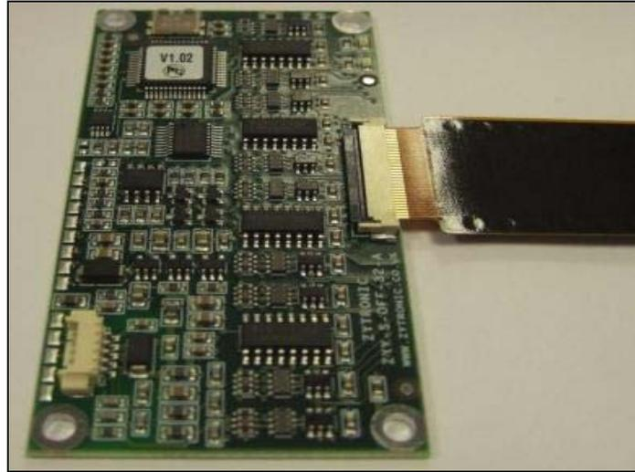
**Figure 11:** Push down locking bar on ZIF connector to lock flexi tail in place
