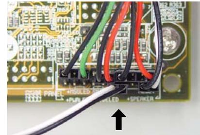
Connect the female ATX power lead from the Slot Adapter to the motherboard's power switch connection (often marked "PWRSW", "PWSW", or "PWBT").
