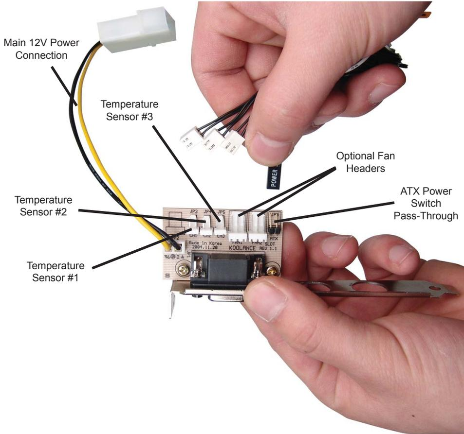
There are 5 main internal connections to the Slot Interface card which will be made. The cooling system can appear to operate without some of these connections, but hardware safety features or temperature monitoring on affected channels will be disabled.
