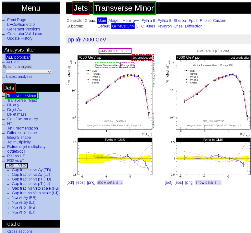
Figure 10: Snapshot of an MCPLOTS page, to serve as an illustration of web page labels. Most label items are produced by processing the file $WWW/mcplots.conf . Section 4.4 discusses changes of $WWW/mcplots.conf , using the text encased by coloured boxes as examples.
