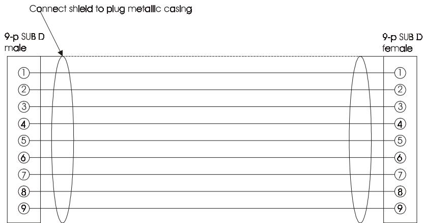
Wires min 0.22 mm<sup>2</sup>, max cable length 3m.
