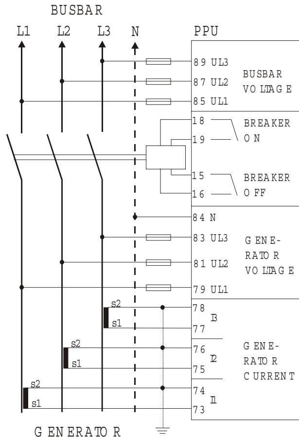
**Notes:** The neutral line (N) connection is not necessary for correct measurement. 3-phase without neutral is also possible.
