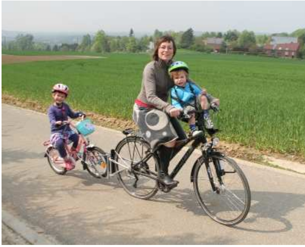
Photo 22: A child's seat in front and a hitch for hooking up a child's bike
