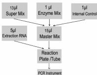
%PCR system without 560nm channel may be to ted with 1µl Molecular Grade Water instead of 1µl IC.
