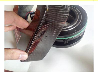
Locate the 3pc M5 mounting bolts (The larger copper bolt is for collimation)
