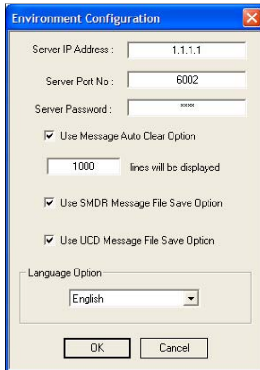
Setup of SMDR / UCD Message Monitor Environment
