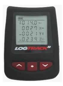
The LogTrackII Data Logger is a very small, thin, low power, easy to use device for measuring barometric pressure, altitude and g-Force data.
