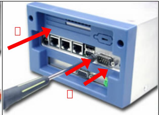
*Fig. 2-41 Place the back panel in position*
