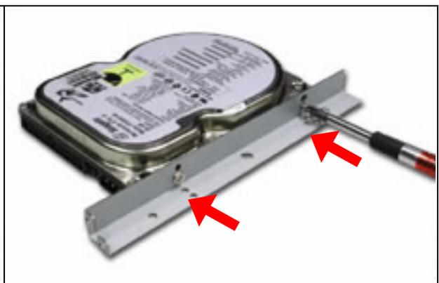
*Fig. 2-26b Fix HDD to the bracket*
