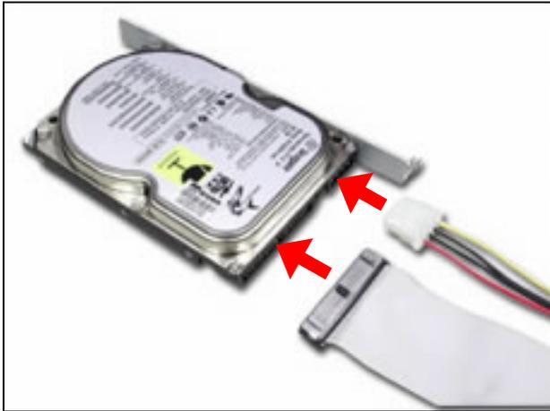
*Fig. 2-27* Connect power and IDE cable to HDD
