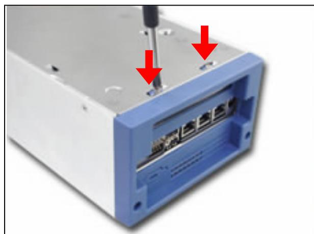
*Fig. 2-5 Press the metal clips on the bottom*
