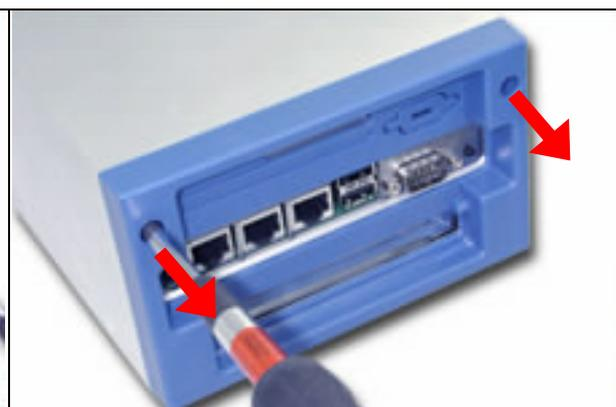
*Fig. 2-4 Take off the screws on back panel*
