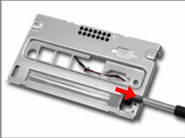
*Fig. 2-38 Remove the original metal bracket*
