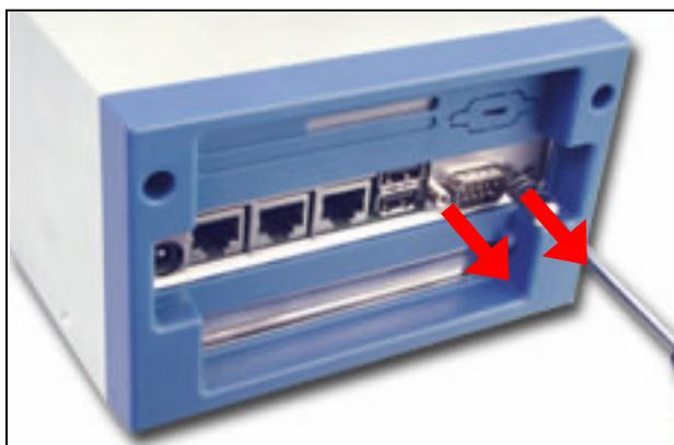
*Fig. 2-3 Remove bolts from COM port*
