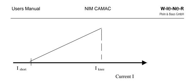
This procedure comes to an end at output voltage U = (nearly) 0 and  $I = I_{short}$ . The parameters  $I_{knee}$  and  $I_{short}$  may be adjusted at R136 and R135.
