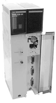
The controller itself is an embedded PC, running Microsoft DOS 5.0. The controller's memory areas and processor are designed to mirror a standard PC.
