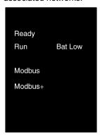
Each indicator is only visible when its associated LED is energized.
