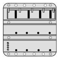
Schneider Electric recommends that the Quantum power supply be installed in the first or last slots in the rack.
