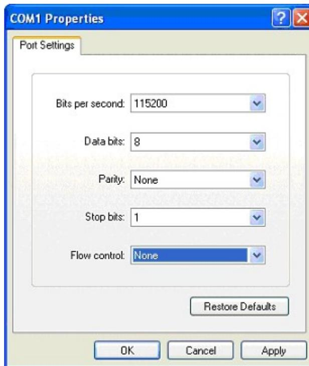
**Fig.4.4 Connection Setting 3 Setting of COM Port**
