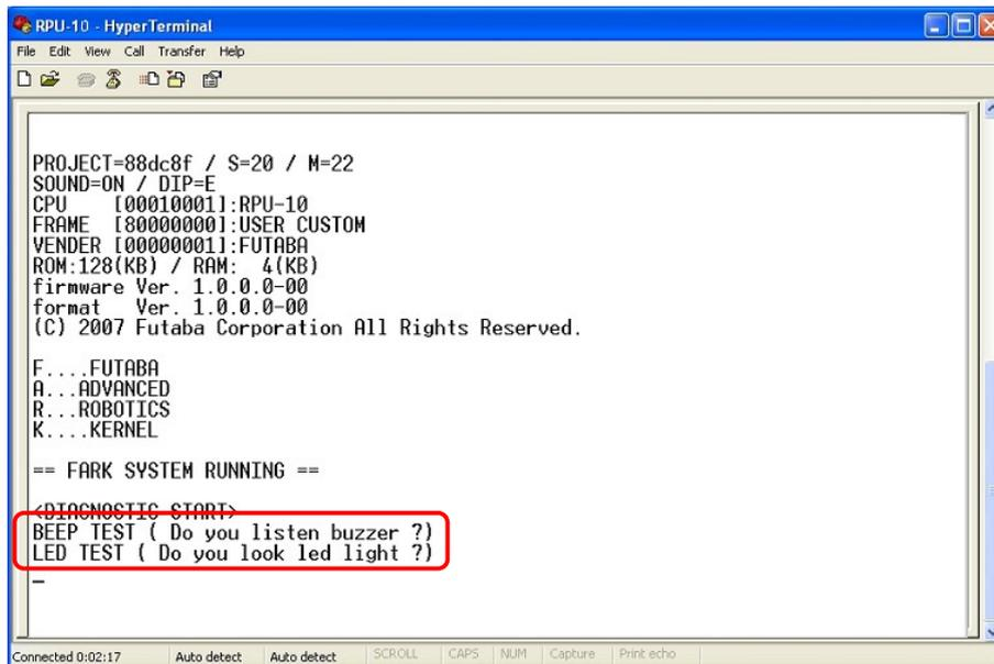
Fig.4.6 Testing of Buzzer and LEDs
