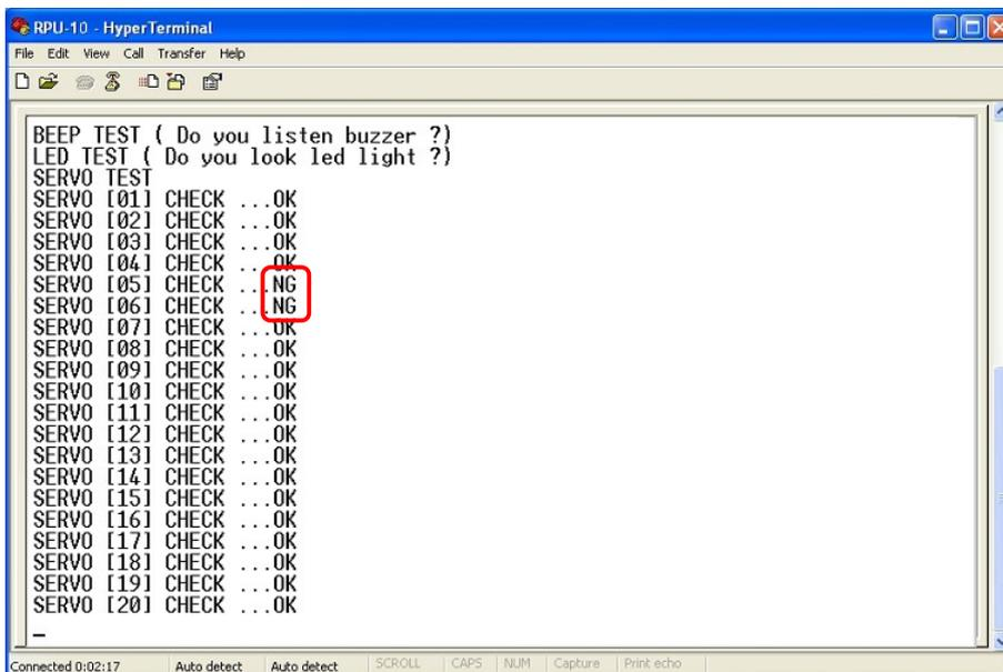
Fig.4.8 Window of Servo Checking(Sample of Connect Failure)
