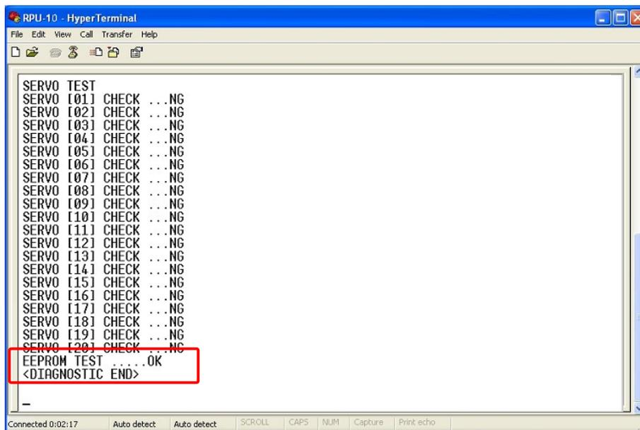
Fig. 4.9 Termination of EEPROM TEST and Self-Diagnosis
