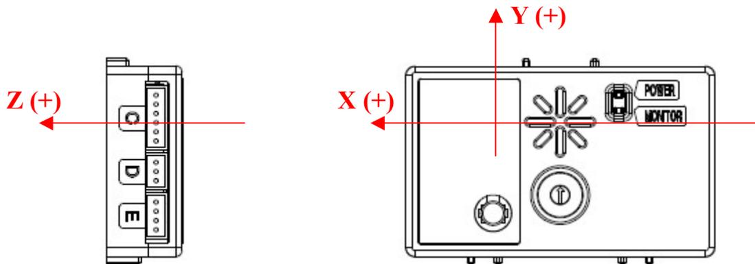
Fig. 2.2G Sensor on RPU-11
