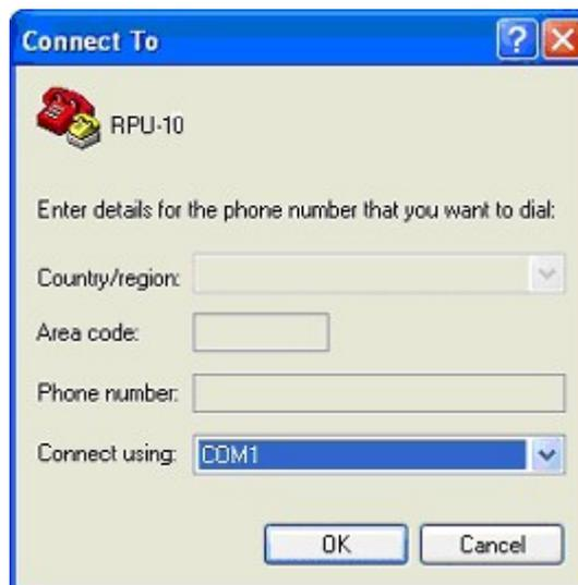
Fig. 4.3 Connection Setting 2 Select the COM Port
