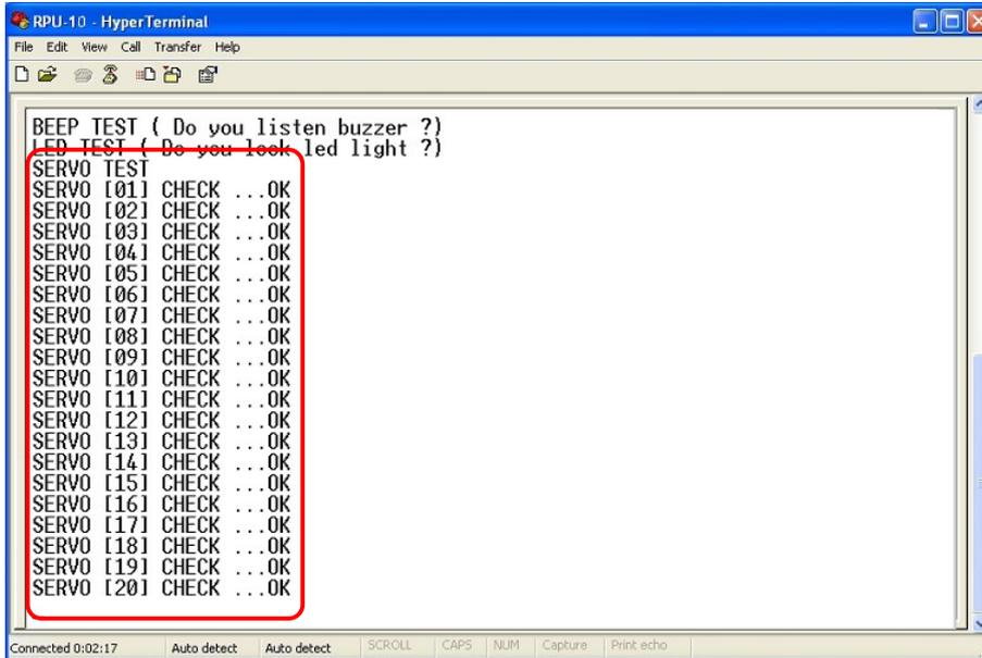
Fig. 4.7 Servo Checking(Connection of all servos is OK)
