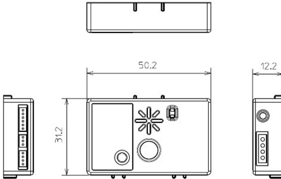
Fig. 5.1 Dimensions of RPU-11 (Unit: mm)
