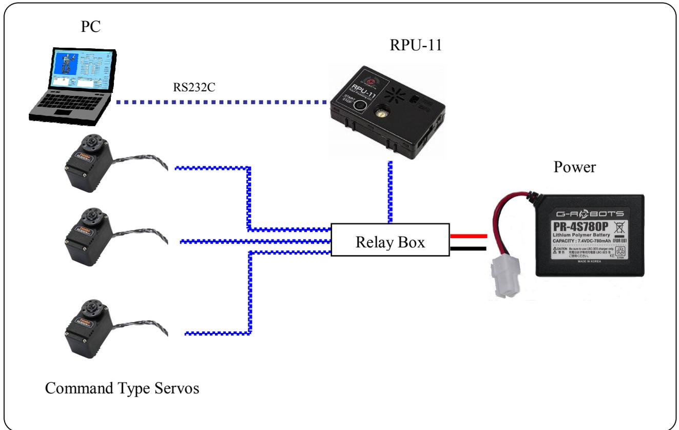
Fig. 3.1 Sample of System Configuration
