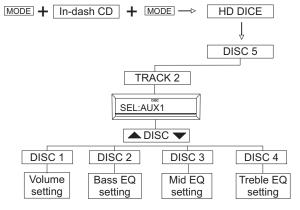
Making the Adjustments. While listening to the auxiliary device, the next/previous buttons adjust the volume (gain), bass, mid and treble. DISC 1-4 modes select what adjustment the next/previous buttons perform. See the illustration for details.
