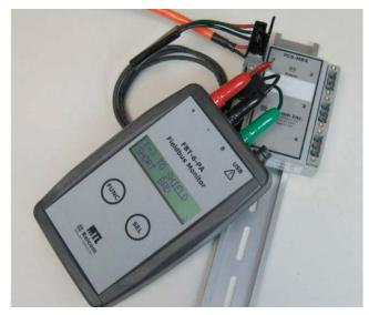
The address (in decimal and hexadecimal) and signal level of each device on the segment is displayed in turn by pushing the "SELECT" button. The first device shown will be the Master. By default, measurements greater than 150mV are OK. If a device leaves the segment, a "-" is displayed; if a device is added it shows "+".
