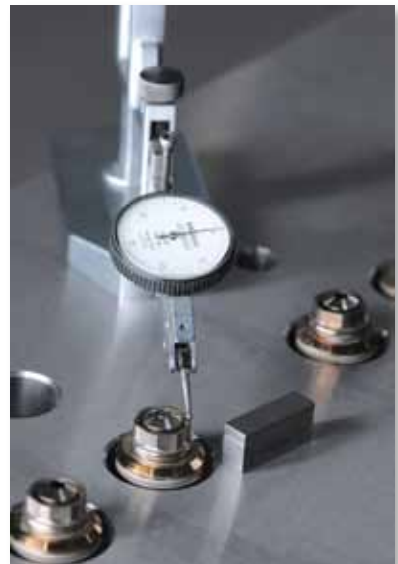
Figure 12-26 Checking Nozzle Tip Height
