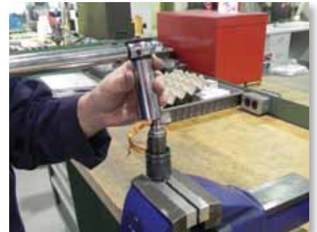
Figure 12-23 Torquing gate seal onto nozzle
