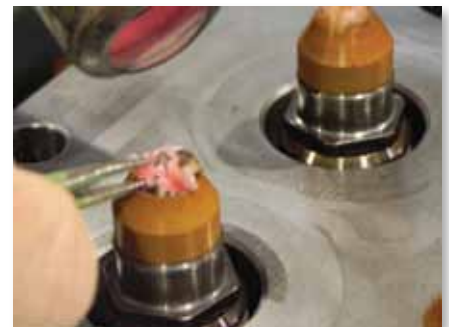
Figure 12-24 Cleaning Insulator Cap
