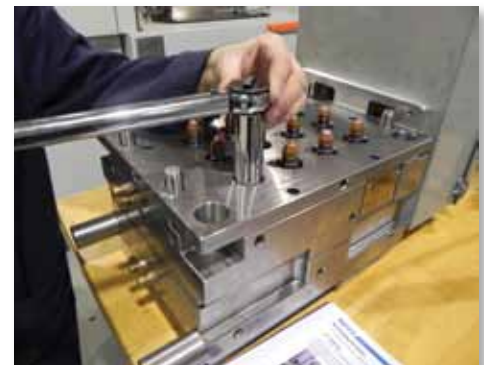
Figure 12-20 Loosening Gate Seal
