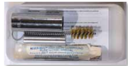
Figure 12-19 Tool Kit for Gate Seal Maintenance
