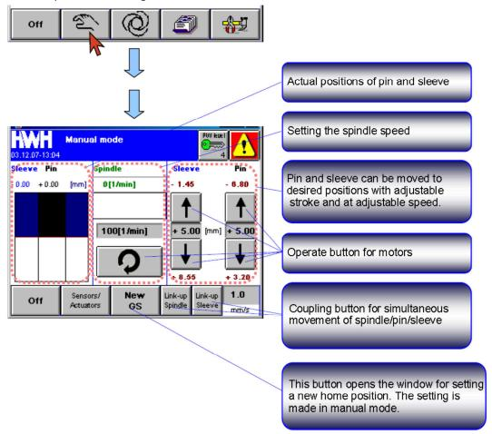
In order to set the correct home position, the welding tool parts must be the level as shown:
