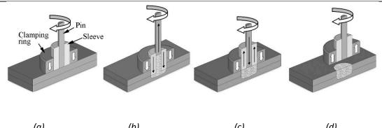
**Welding Process overview:** *a) clamping and spindles rotation, b) sleeve plunges into the sheets while pin moves upwards, c) sleeve retracts back, and d) withdrawal of welding head*
