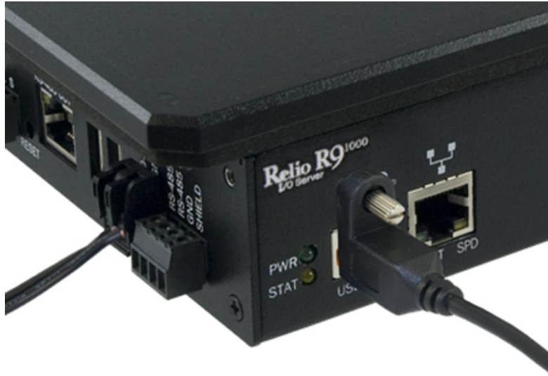
Figure 30. Type B USB Device Connector
