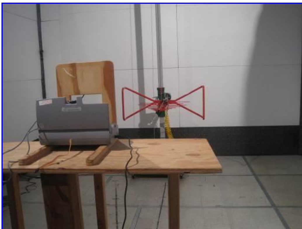
Radiated Emission Set up (<30MHz) – Rear View
