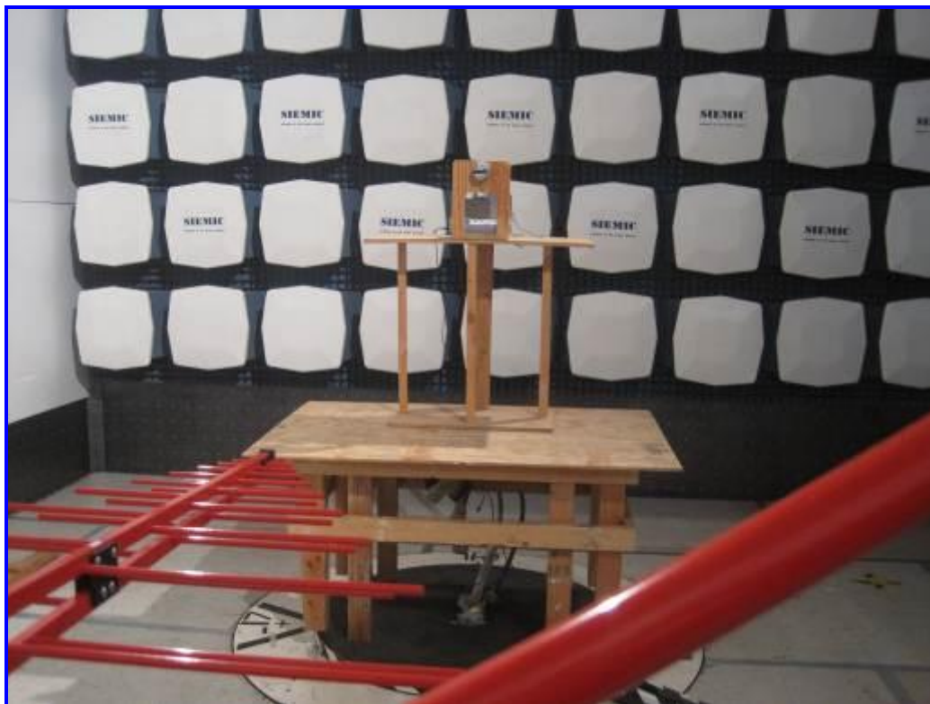
Radiated Emission Set up (<30MHz) – Front View
