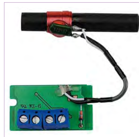
Figure 3. A DCF77 receiver module is used for precise time synchronization. This module is based on the proven Temic DCF77 receiver IC.
