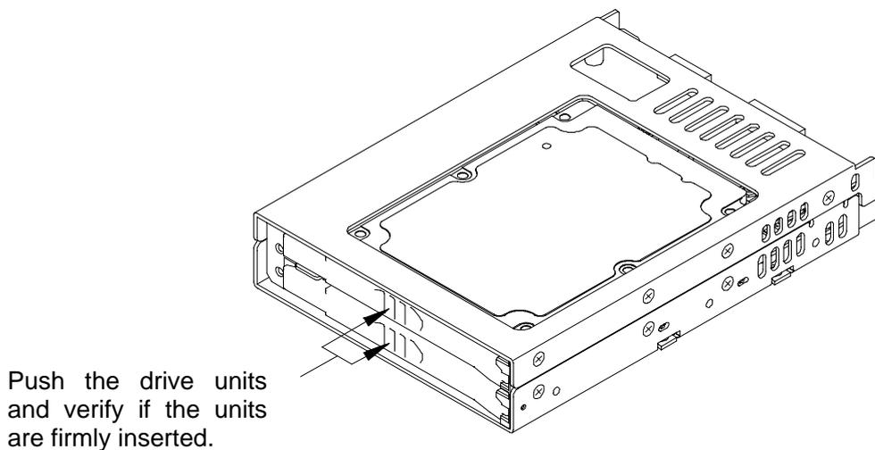
Push the drive units and verify if the units are firmly inserted.
