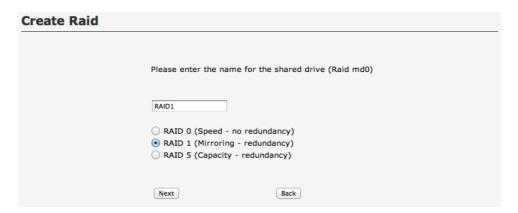
**Please note:** RAID 0 and RAID 1 require a minimum of two hard disks, the minimum for RAID 5 is three hard disks and RAID levels 6 and 10 require four harddisks.
