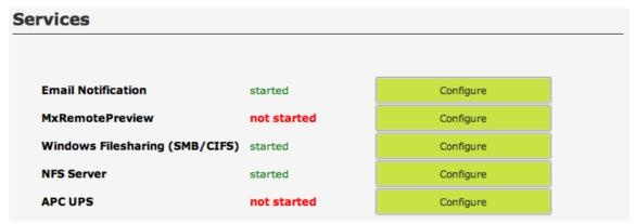
You can configure detailed settings for each system service via the button ,Configure'.
