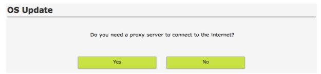
In case your site uses a proxy to connect to the internet, click on the ,Yes' button and specify the site-specific proxy settings, as shown below. After clicking on ,Save', the specified proxy will be used in order to find a firmware update. In case there is a more recent firmware version available, it will be automatically downloaded onto the server appliance.
