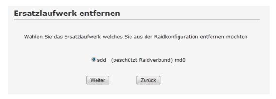
Select the hard disk that you want to unassign from the list and click on ,Next' – the hot spare will be unassigned and you can now find another use for it – as a member disk of a to-becreated RAID or as a hot spare disk of a another RAID, for instance.
