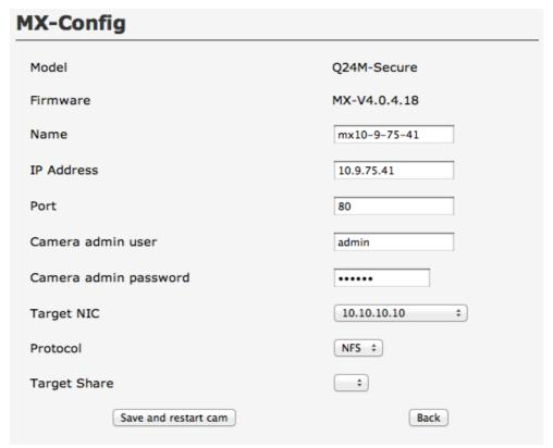
After having made the configuration changes click on 'save settings and restart camera'. Depending on the camera model it may take up to a minute until the camera will have restarted and be available in the overview. Click on 'back' to return to the MX configuration menu.
