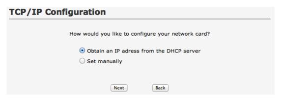
In case you have selected ,DHCP', you are done with network configuration – click on ,Reboot server' in the next menu to apply the settings. Otherwise, for manual network configuration, enter the IP address, the subnet mask and the gateway and then save your settings by clicking on ,Save'.
