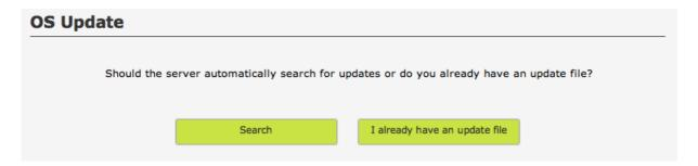
• **Search:** The easiest way to update the firmware is by automatic search. By clicking on the ,Search' button, the system will establish an internet connection to a Exus Technology server and check whether more recent firmware, than the one that is installed on your server appliance, is available.
