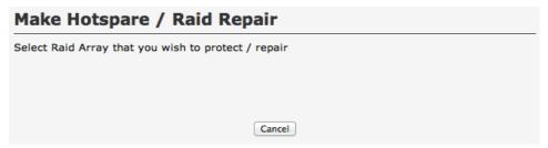
The selected hard disks are now assigned to and reserved for this particular RAID and will be used as spare drives as soon as a component hard disk of this RAID fails or is removed.
