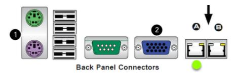
PS/2 connectors for mouse and keyboard are located at the very left side (1) and the blue connector for a VGA monitor can be found at position (2), to the left of the two Ethernet ports, which are located at the very right side of the connector panel.
