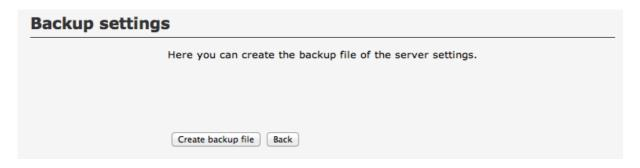
Here's how its done: First click on the button, Create backup file'. The QStor QMX server appliance generates a backup file with all system settings and lets you download this file. This file is always named, serversettings.tar.gz' and is in the GZIP format. Clicking on the file name will start the download process.
