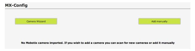
2. You can conveniently configure a new camera via the camera wizard, by clicking on the button ,Camera Wizard' in the ,MX Config' window. After clicking on ,Next', the server begins to scan the network for newly added cameras. This operation may take several minutes.
