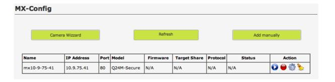
You can modify camera settings at any time by clicking on the gear icon in column ,Action'. Column ,Action' also allows you to do other things: Clicking on the ,Play' icon will show you the live feed of the camera in a new window and clicking on the red circle will manually start recording. You can also delete a camera that is no longer needed by clicking on the broom icon.
