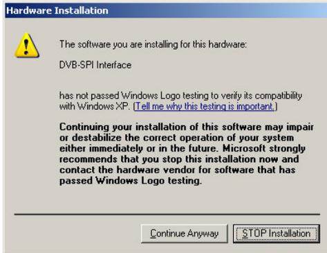
Click the CONTINUE ANYWAY button. The system sets a Restore point then completes the installation. The Completing found new hardware screen appears.
