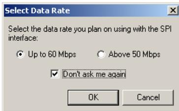
Click “Up to 60 Mbps”, check “Don’t ask me again” then click OK. If you have the LVDS to USB adapter plugged into the back of the DM1010, and the DM1010 is tuned to a channel with Sync, EQ, and TOV lock lights lit, and the Transport Stream output is enabled IE “TS+” on the DM1010 display the you should see the TSReader Professional screen appear with the PID table decoded and an active PID list displaying percentage of use of total bandwidth of each program stream.
