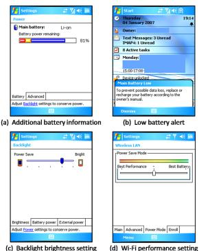
Figure 2. Battery interfaces on the HTC Wizard phone
