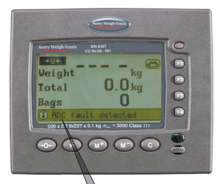
Example: This error message shows that there is an analogue/digital conversion fault. Replace the Operator Display Panel or the scale base to correct this.
