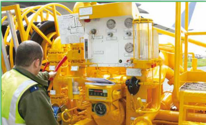
This application shows uploading fuel into an aircraft with the icountPD in use to monitor as a 'go/no go' device.
