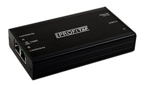
The ProfiShark 1G is a handheld, Plug and Play device dedicated to inline gigabit monitoring. It facilitates in-field traffic capture and troubleshooting. The ProfiShark 1G is equivalent to a 10/100/1G aggregator TAP and two 1 Gbit/s NICs. All-in-one in a pocket-sized box, the only additional hardware required being a laptop with a free USB 3.0 port.
