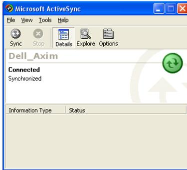
Before installing the Prosurv software, make sure that your Microsoft ActiveSync® program is running, and that it displays “Connected” and “Synchronized”.
