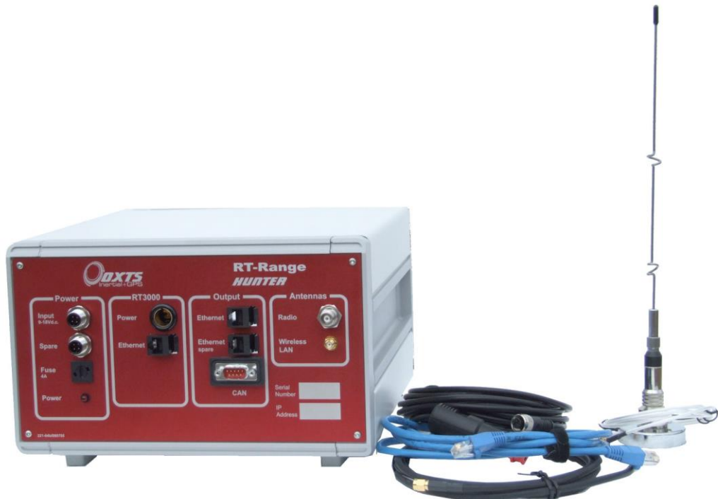
Figure 3. Image of RT-Range Hunter with Components
