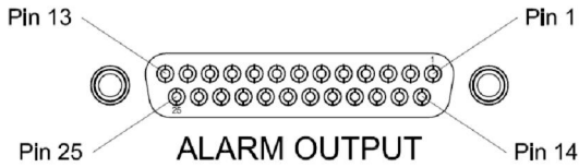
Figure 5.10 PerformMAX IQ Power Supply Alarm Output Connections
