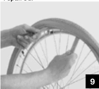
Remove the rim assembly (tyre and inner tube), repair or replace the inner tube, reinsert in the tyre and reposition the assembly on the rim.
