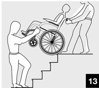
The wheelchair must not be lowered until the last step has been passed and the chair is clear of the stairs.
