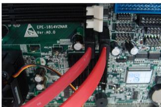
Step 2: Please connect the SATA data cable to the SATA connector on the board.
