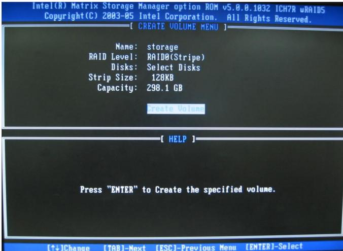
F: Choose the serial optional value for RAID array via upper or down arrow and press <Enter> to confirm and enter the next region. The optional value ranges between 4KB and 128 KB and increases in fold. The selection of serial value is based on the operating method of the driver. There are some recommended options: RAID0-128KB RAID10-64KB RAID5-64KB
