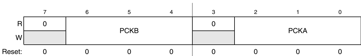
Figure 26-5. PWM Prescale Clock Select Register (PWMPRCLK)
