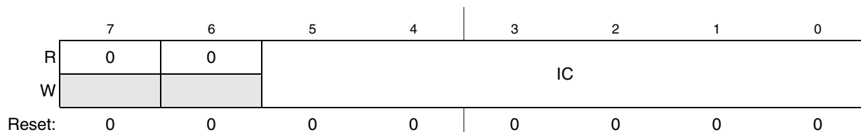
Figure 24-3. I 2 C Frequency Divider Register (I2FDR)
