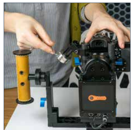
Figure 5. Adjusting weights on the antenna (step 10)
