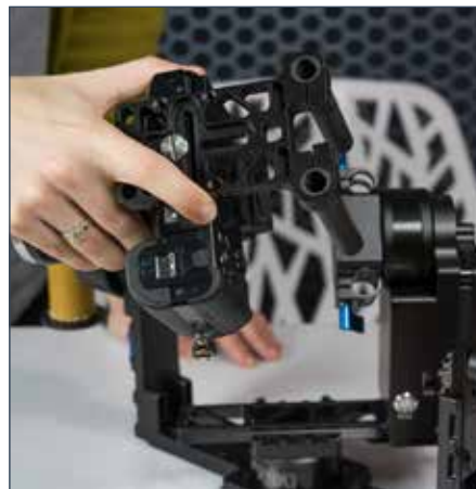
Figure 4. Inserting baseplate rods into the clamps (step 4)
