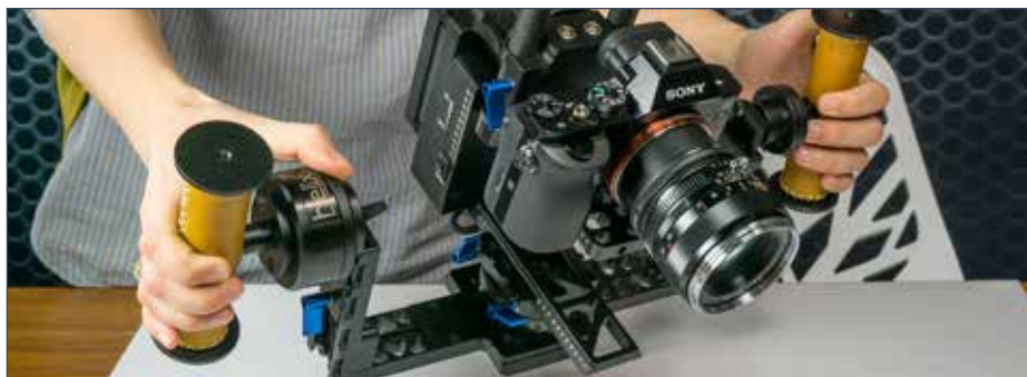
Figure 8. Rotating the camera forward using a thumb on the inside of the tilt motor (step 2)
