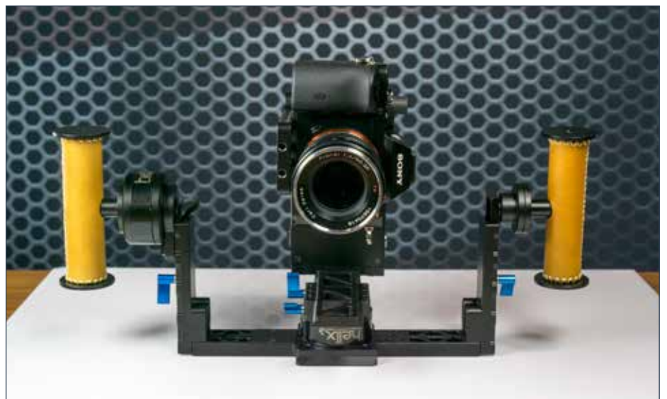
Figure 6. Camera adjusted so that it stays oriented with camera sideways (step 7)
