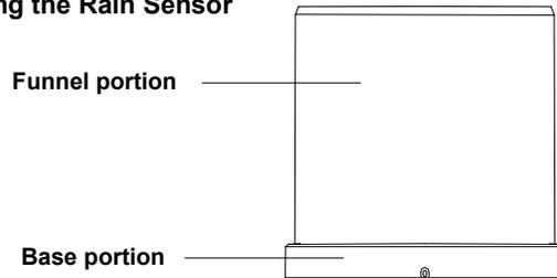
For accurate results, the rain sensor should be securely mounted onto a horizontal surface at least 1.0 metre above the ground and in an open area away from trees or other coverings where rainfall may be reduced causing inaccurate readings. Placing the gauge extremely high is generally not a good idea as you may need to periodically clear debris such as leaves, spider nests etc.
