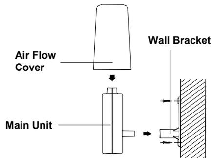
An ideal mounting place for the thermo-hygro sensor would be the outer wall beneath the extension of a roof, as this will protect the sensor from direct sunlight and other extreme weather conditions.
