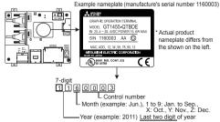
The production date of the optional replacement battery can be confirmed by the lot No. marked on the nameplate (label) affixed on the battery.
