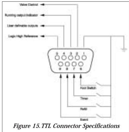
Figure 15. TTL Connector Specifications
