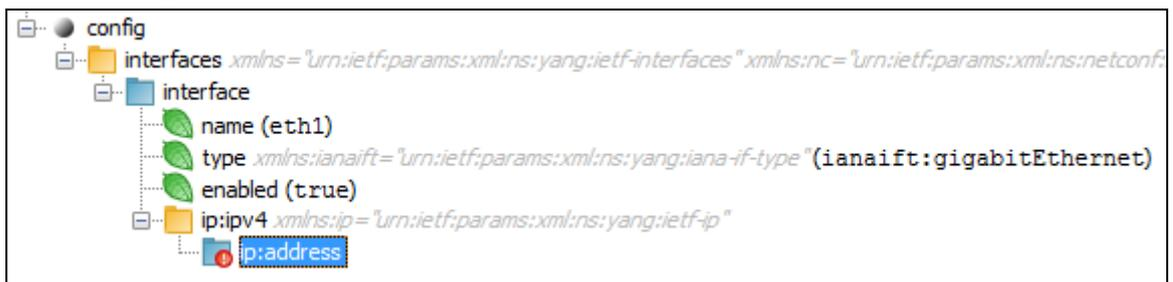
Figure 78: New `ip:address` list element in the configuration tree
