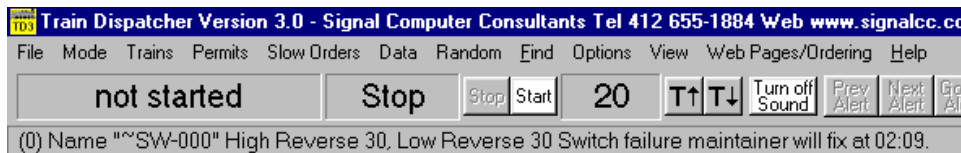
Figure 10 - Switch Status Line
